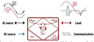
Pure sine wave at the output and ideal power factor at the input are achieved without pumping any energy from the DC source.
