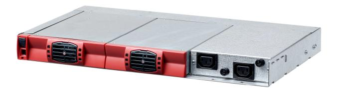
The TSI is designed according to the golden rules of **True Redundant Systems**. One of the most important features is the disconnection capability. A TSI converter has no less than 3 disconnecting levels in series (i.e. electronics, relay and fuse) on its DC power port as well as an optical isolation on the double communication bus.
